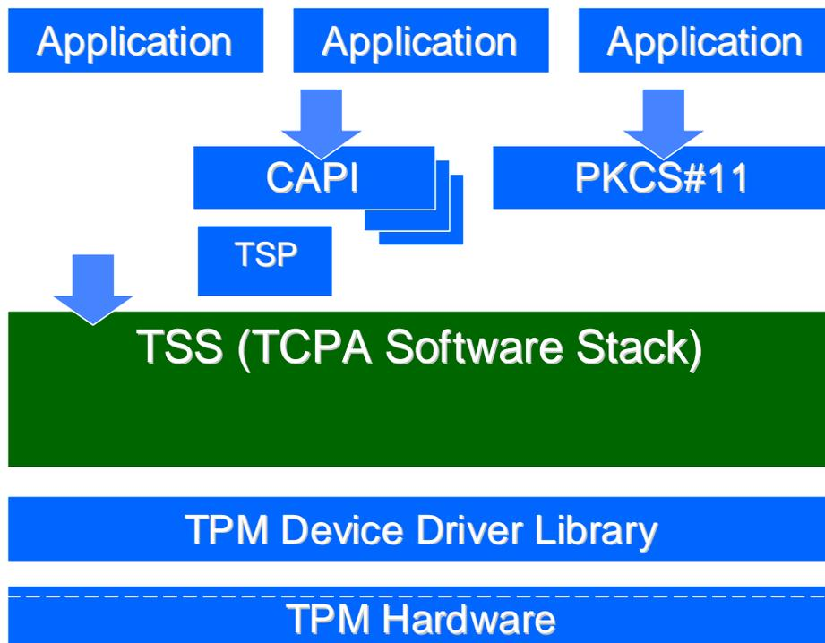
Applications can utilize the TPM either through the MS-CAPI standard interface, or by directly implementing a communication interface with the TSS, especially for certain TCPA functions that may not be supported by MS-CAPI.
