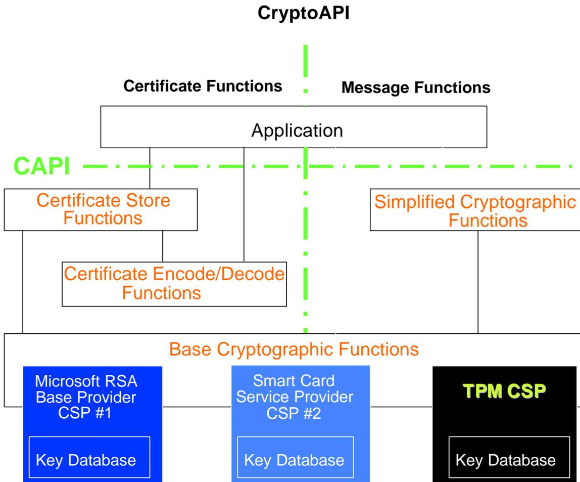
The TPM CSP provides an interface between the CAPI and the TSS. Since the scope of the TSS is much broader than that of the CAPI, several TSS capabilities are not accessible through the CAPI. Such advanced capabilities are directly accessed through the TSS – applications needing such capabilities have to directly talk to the TSS.
