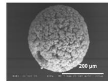
SEM picture of a mixed oxide prepared with a spherical activated carbon.
