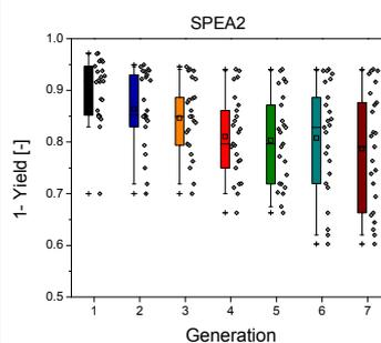
Evolution of the objective function (1 - conversion of NO to N<sub>2</sub>).
