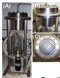
Images of the 49 parallel channel reactor setup: (A) side view on the complete setup, (B) top view on the open reactor (C) closed reactor.
