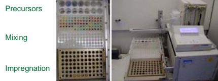
Fig. 1: ABIMED liquid handling robot for automated precursor mixing and impregnation of activated carbon particles.
