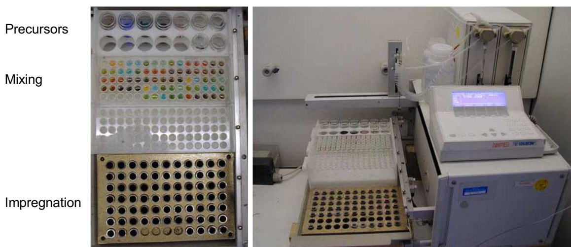
Figure 4.3: ABIMED liquid handling robot robot for automated precursor mixing and impregnation of activated carbon (Martinez Joaristi, 2007).
